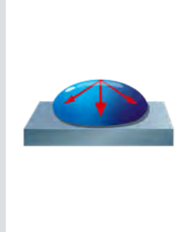
Medium Surface Energy PET, ABS, PVC (rigid), polycarbonate, polyimide, polyurethane (rigid), acrylic (PMMA), most paints and coatings
