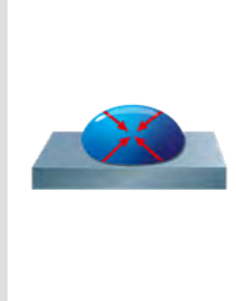
Low Surface Energy Polypropylene, polyethylene, TPO, PTFE, acetyl, PBT, polystyrene, EPDM rubber, some paints and coatings (PVDF)
